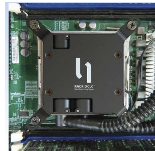
CoolIT systems - Direct Contact Liquid Cooling
